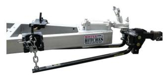
One approach is to fit a Weight Distribution Hitch (WDH) between your vehicle's towbar and the trailer. This picture shows a typical setup that involves using tension bars connected to the tow bar coupling to transfer weight (down-force) of the trailer as an up-force to the rear vehicle chassis resulting in a load transfer off the rear axle and onto the front axle. The resulting up-force will cause the
